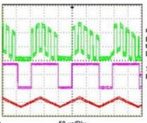
modulated, pulsed and triggered Diode current
